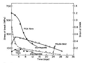
Figure 2 In vitro test on the fibres of poly(amide-ester) and poly(glycolic ester) in Ringer solution. Variation of stress (---) and strain (---) with time
