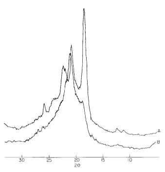
Figure 4 X-ray diffraction diagrams for poly(amide-ester) film POLEA 3612: A, after degradation; B, before degradation
